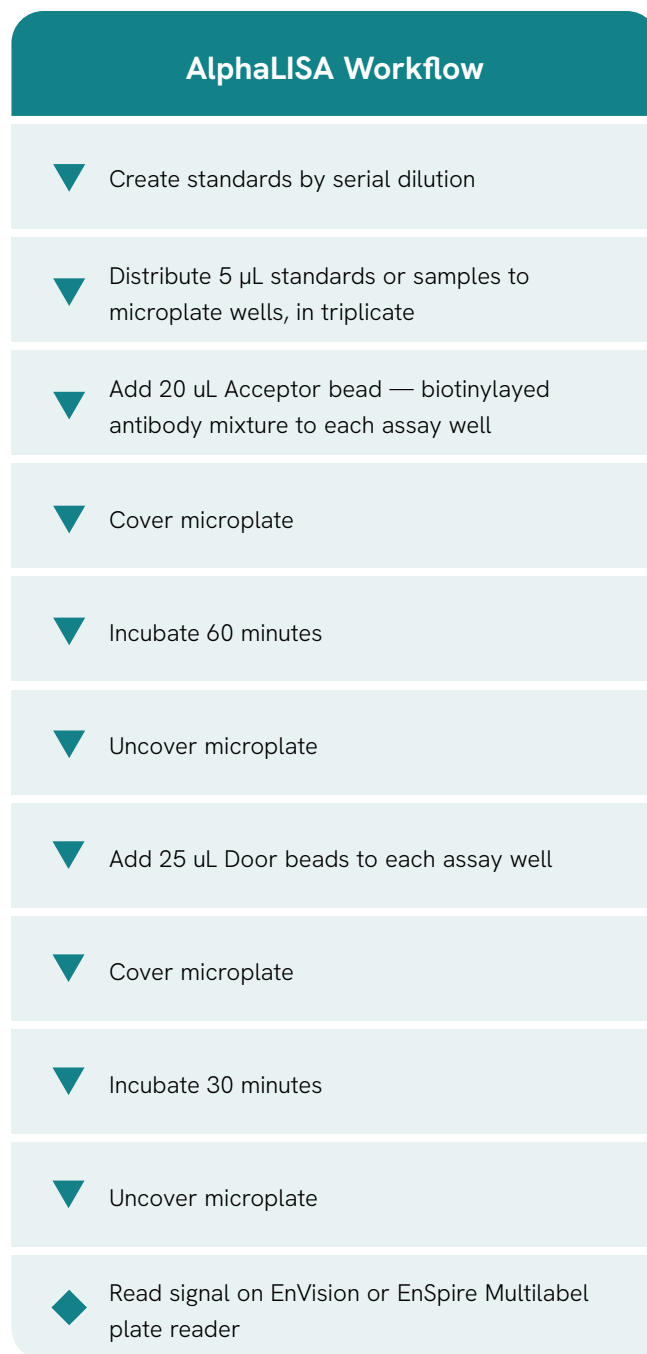
Figure 1: The AlphaLISA assay workflow is depicted above. All the steps outlined were performed by the JANUS AlphaLISA Workstation and an EnVision reader, as well as manually.
